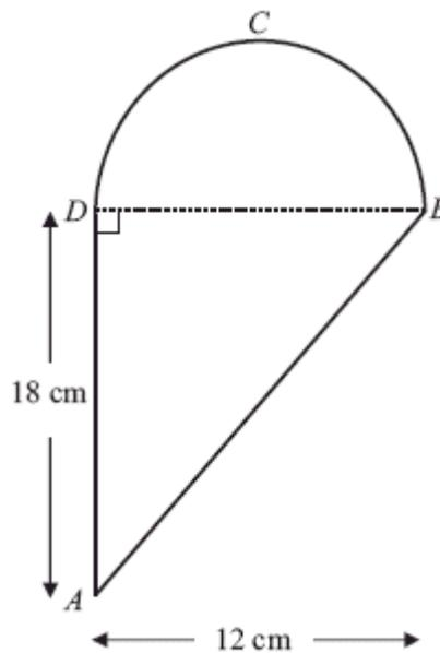
A uniform lamina  $ABCD$  is made by joining a uniform triangular lamina  $ABD$  to a uniform semi-circular lamina  $DBC$ , of the same material, along the edge  $BD$ , as shown in the diagram above. Triangle  $ABD$  is right-angled at  $D$  and  $AD = 18$  cm. The semi-circle has diameter  $BD$  and  $BD = 12$  cm.
