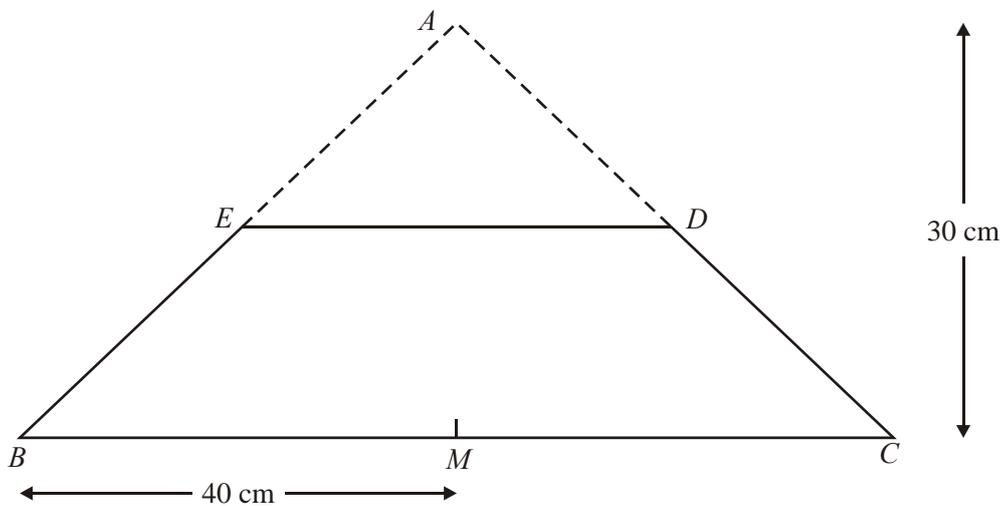
A uniform plane lamina is in the shape of an isosceles triangle  $ABC$ , where  $AB = AC$ . The mid-point of  $BC$  is  $M$ ,  $AM = 30$  cm and  $BM = 40$  cm. The mid-points of  $AC$  and  $AB$  are  $D$  and  $E$  respectively. The triangular portion  $ADE$  is removed leaving a uniform plane lamina  $BCDE$  as shown in the diagram above.
