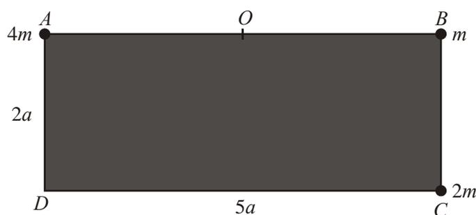
A loaded plate  $L$  is modelled as a uniform rectangular lamina  $ABCD$  and three particles. The sides  $CD$  and  $AD$  of the lamina have lengths  $5a$  and  $2a$  respectively and the mass of the lamina is  $3m$ . The three particles have mass  $4m$ ,  $m$  and  $2m$  and are attached at the points  $A$ ,  $B$  and  $C$  respectively, as shown in the diagram above.
